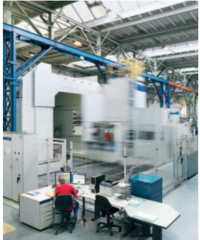
Dörries Scharmann, Heavyspeed CNC Milling Machine Centric table load: 23'000 kg, spindle stroke: 1000 mm
