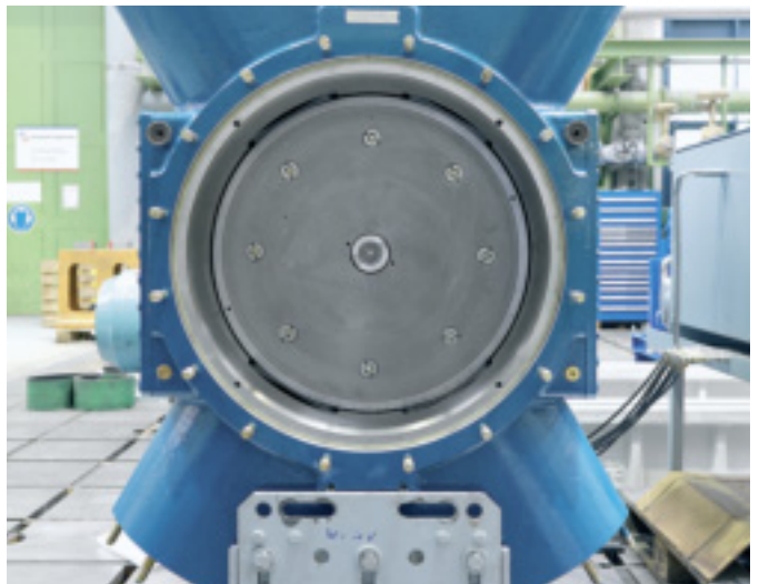
Easy access to piston and cylinder liner
