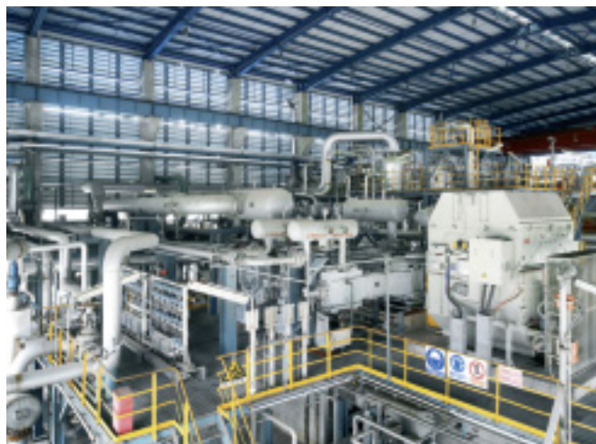
LDPE compressor train: Process Gas Compressor and Hyper Compressor at 3'100 bar by Burckhardt Compression – the global technology leader in the reciprocating compressor world
